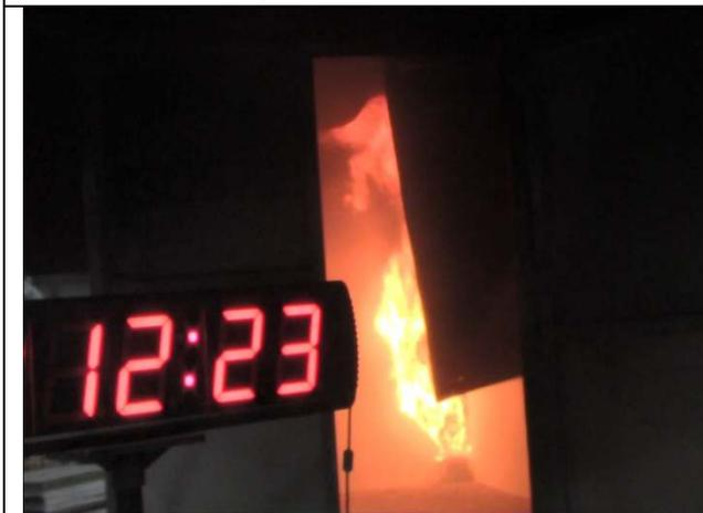
Figure 3. The sample on the right side of the ceiling began to fall off (12min:23s)
