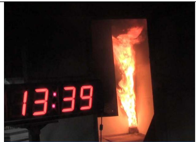
Figure 4. The sample in the middle of the ceiling a began to fall off (13min:39s)
